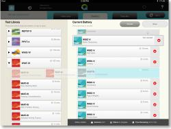
The Battery Details at the bottom of the screen show you where you are within your battery, as well as the estimated time remaining. You can edit your battery at any time; however, completed subtests are not editable. You can re-order subtests on the right side by pressing and holding, and then dragging them to the desired order. You can also delete a subtest by tapping the red X on its bar. After all of your edits have been made, tap the Save button to execute the changes.
